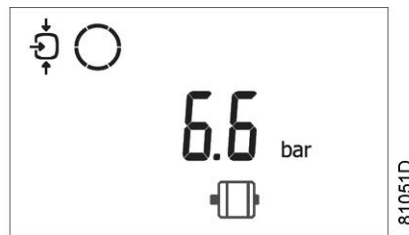
Main screen with shut-down indication, motor overload
